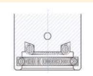
The butt contact is used in the current test of a general-use terminal board. Even more stable energization is ensured by energizing the two directions of the upper and lateral sides using two coil springs for the screw head.
