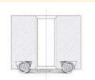
The butt contact is used in the current and breakdown tests of the pre-shipment inspection of the IGBT. Stable energization is ensured by multipoint contact, and damage to the terminal block of the IGBT can be minimized.
